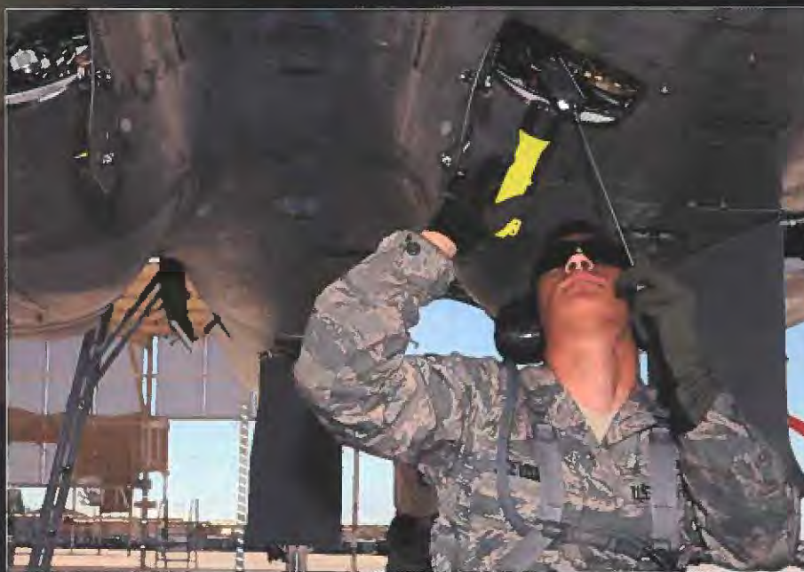
Senior Airman Pedro Acevedo of the 159th Fighter Wing Maintenance Squadron inspects the Airframe Mounted Accessory Drive of an F-15 Eagle fighter jet as part of the pre-flight inspection to Luke Air Force Base in Phoenix, Arizona on June 9, 2011. Inspections are key to maintaining a flight worthy aircraft and ensuring the safety of the pilot.
