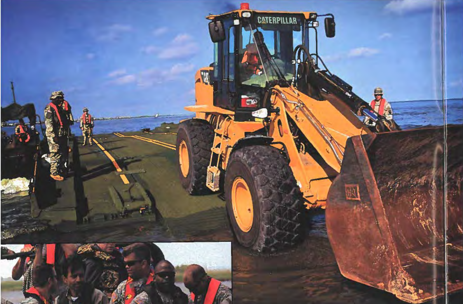
GRAND ISLE, La. – Soldiers of the 2225th Multi-Role Bridge Company, 205th Engineer Brigade, offload a front end loader from a five-panel improved ribbon bridge raft in Grand Isle, La., July 2, 2010. Photo: Spc. Christopher Foster
